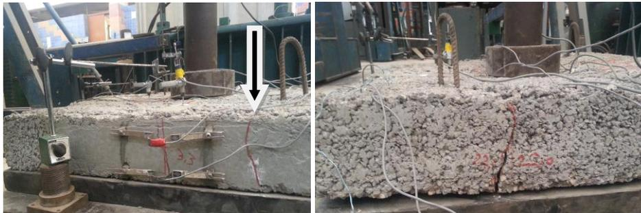
Figure 7. Crack pattern of control slab M1SL1 under central vertical load
