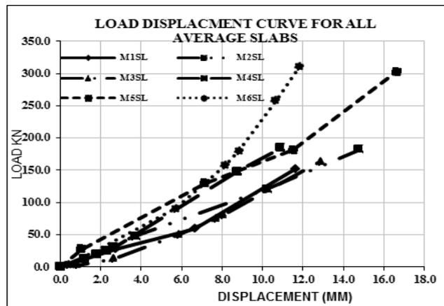
Figure 5. Load-displacement relations for all slab types
