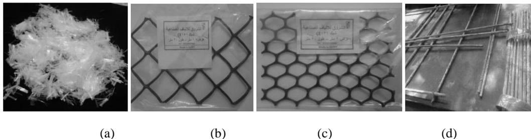
Figure 1. The used strengthening materials: (a) fibrillated polypropylene fibers, (b) geogrid type I, (c) geogrid type II and (d) GFRP bars
