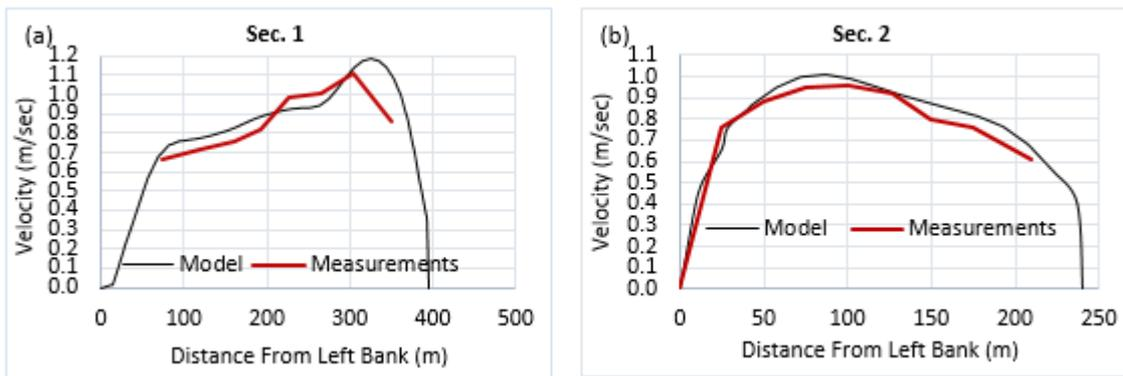
Fig 3. The velocity calibration
