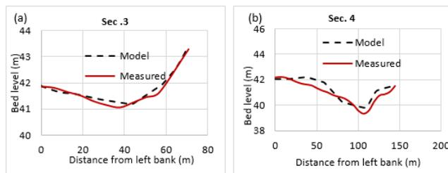
Fig7. The bed level calibration
