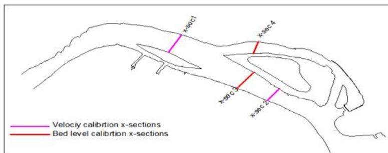
Fig 2. Locations of measured cross-sections in 2006
