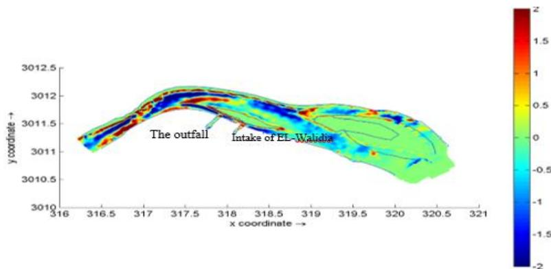
Fig 12. deposition and Erosion from 2015 to 2025 (+deposition, -erosion)
