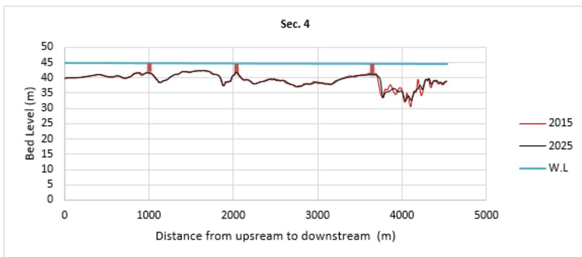
Fig 14. Predicted cross sections of bed level from upstream to downstream
