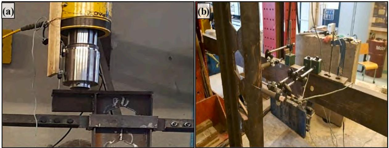
Fig. 7. Arrangement of LVDTs of Groups II&III: (a) Horizontal LVDTs of Groups II&III; (b) Vertical LVDT of Groups II&III.
