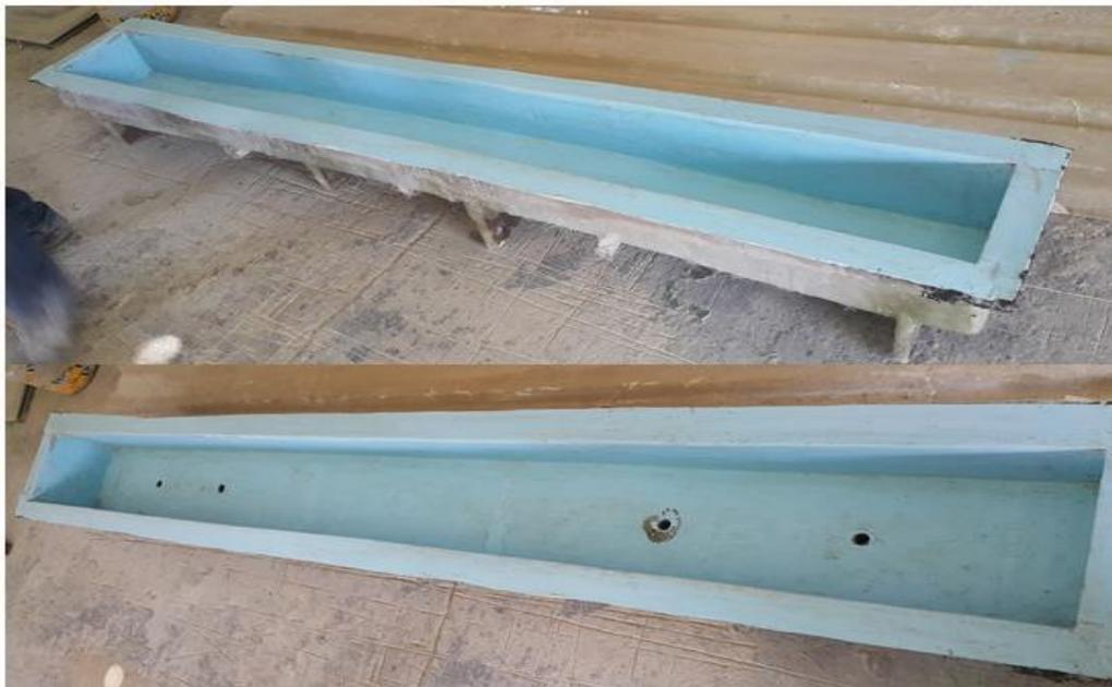
Fig. 1. Mold of proposed composite sleeper
