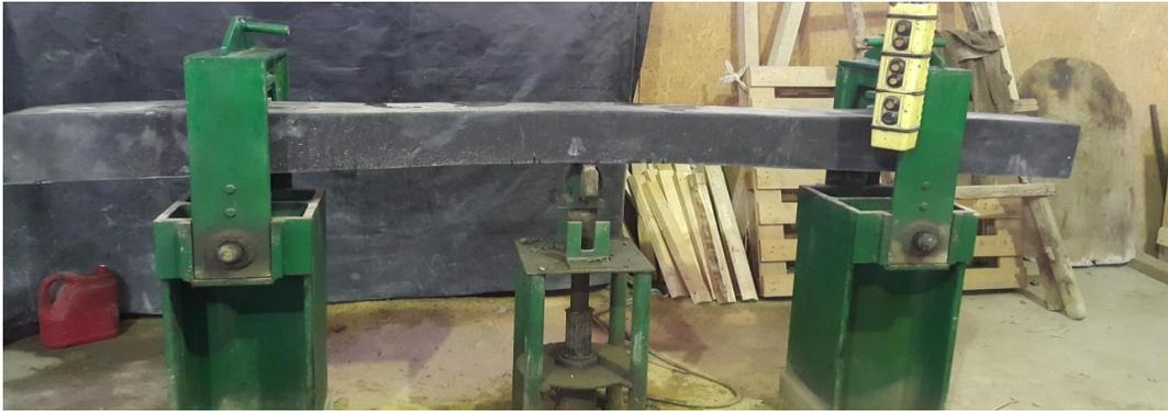
Fig. 9. Sleeper (S<sub>10</sub>) under 72 kN static loading of the sleeper center section
