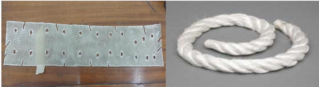
Fig. 3. Used fiber glass laminate and rope in sleeper reinforcement
