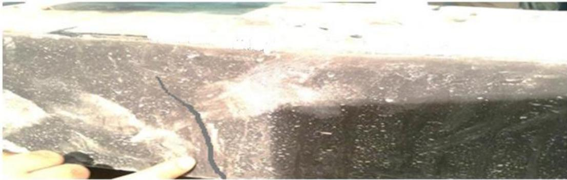
Fig. 10. Failure mode of sleeper  $S_{10}$  under static load on rail seat section
