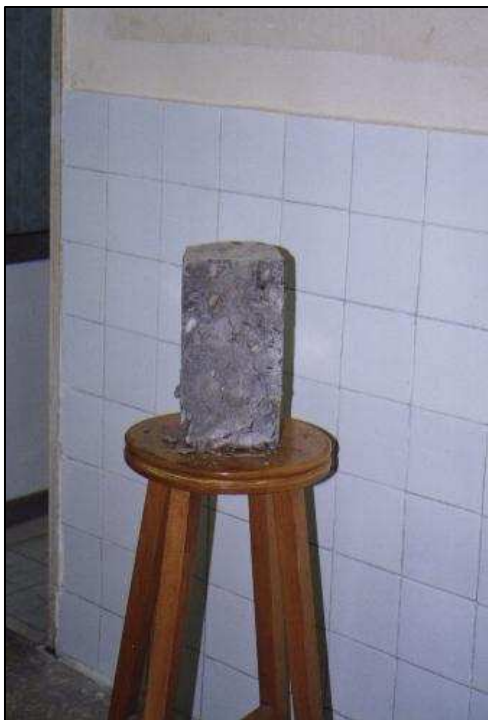
Figure (2) Concrete specimens (8) and (20) after failure
