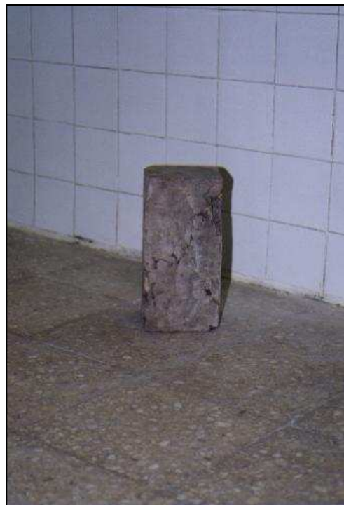
Figure (2) Concrete specimens (8) and (20) after failure
