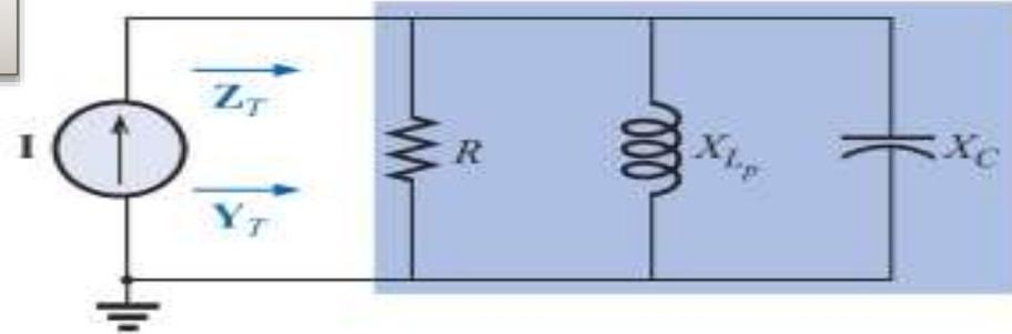
➤ The cutoff frequencies  $f_1$  and  $f_2$  can be determined using the equivalent network shown in the figure:
