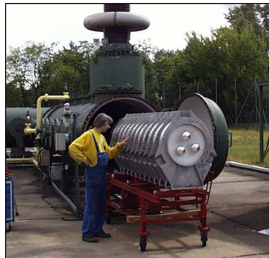
Figure 4: Example of test setup for disk insulators
