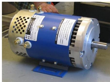
The dc motor is basically a torque transducer that converts electric energy into mechanical energy. It consists from **Stator** that contain the field flux and **Rotor** (armature) that contains the windings. DC motor is modeled as a circuit with resistance  $R_a$  connected in series with an inductance  $L_a$ , and a voltage source  $e_b$ , representing the back emf (electromotive force) in the armature when the rotor rotates as shown in Fig. 19.
