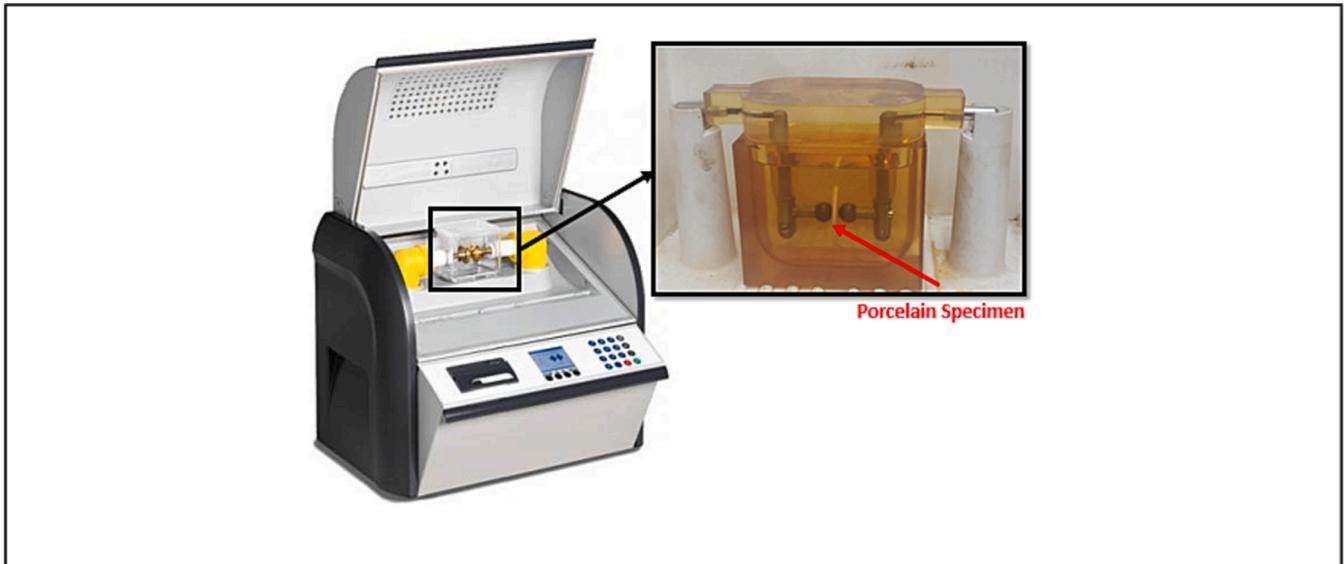
Fig. 8. AC breakdown tester with the tested porcelain specimen.
