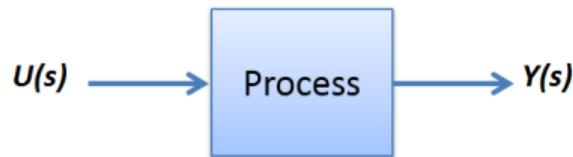
$$G(s) = \frac{\text{numerator}}{\text{denominator}} = \frac{\mathcal{L}[\text{output}]}{\mathcal{L}[\text{input}]} = \frac{Y(s)}{U(s)} = \frac{b_0s^m + b_1s^{m-1} + \dots + b_{m-1}s + b_m}{a_0s^n + a_1s^{n-1} + \dots + a_{n-1}s + a_n} = \frac{p(s)}{q(s)} \quad (n \geq m)$$
