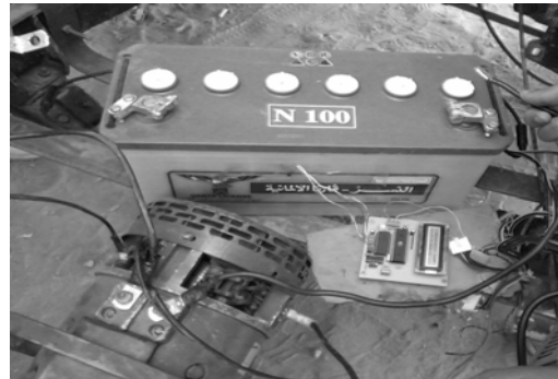
Figure 9: Practical Setup for measuring Temp. And SOC
