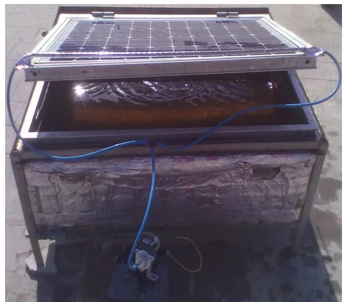
Figure 2: View of PV module with water film cooling system.
