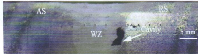
(c) \omega = 300 rpm, v = 20 mm/min
