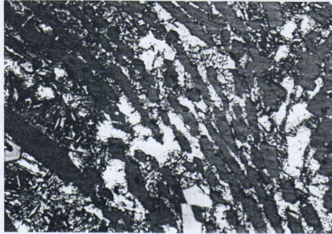
Fig. (6) Microstructure of piston alloy/16 wt.% Ni composite prepared under application Of pressure during solidification.
