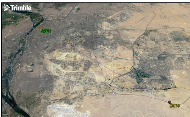
Figure 3. Baseline between SFE1 and base station for kinematic work
