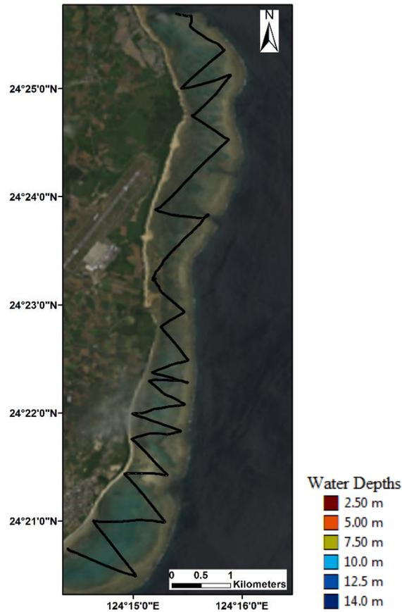
Figure 2-11. Field bathymetry Reference points of the 4<sup>th</sup> study area from echo-sounder.
