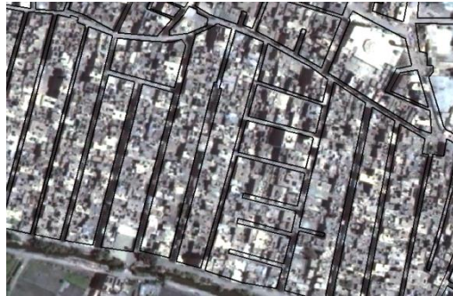
Figure (7): On screen digitizing for QUICKBIRD satellite image for streets.
