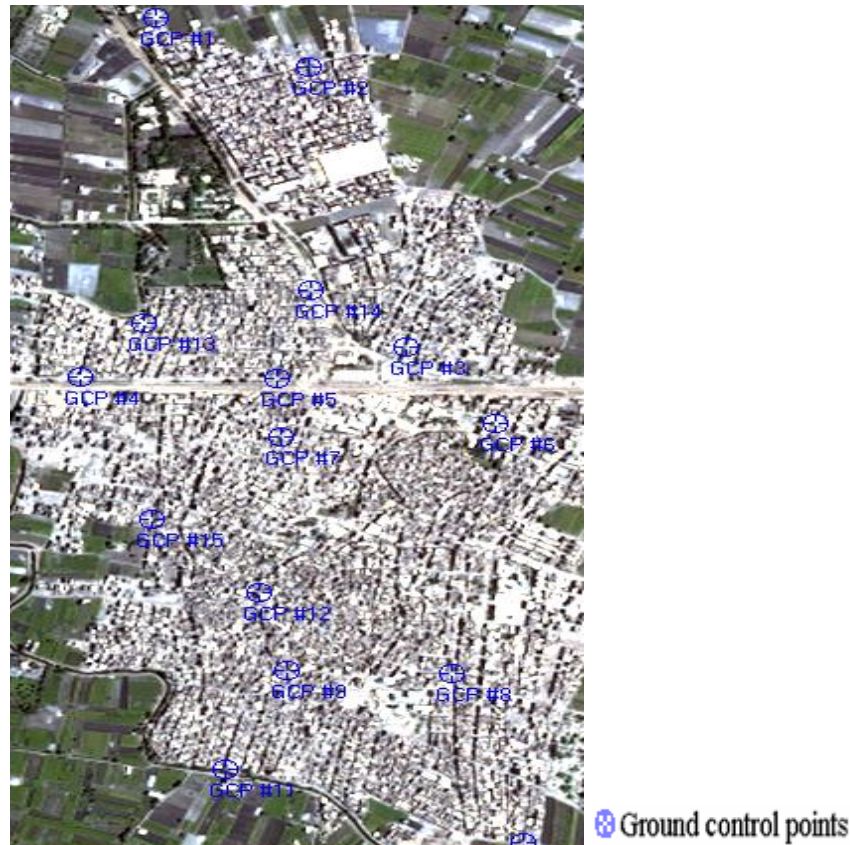
Figure (1): Well observed and distributed GCPs over the area under investigation on QUICKBIRD satellite Image.
